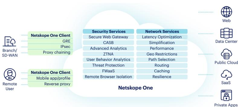
Figure 1: In addition to support for legacy proxies, firewalls, SD-WAN devices, and clientless options, Netskope One Client simplifies steering traffic to Netskope NewEdge.
