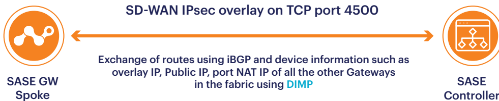
Figure 3: Routes and Device Information Exchange with Controller
