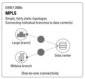
**FIGURE 1-1:** In the one-to-one world, branch offices use MPLS to connect to a centralized location called the data center, where all the applications are hosted.
