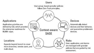
**FIGURE 5-1:** A rich context focused on users, devices, applications, and the associated risks is a necessary ingredient to enable the definition of granular SASE policies.
