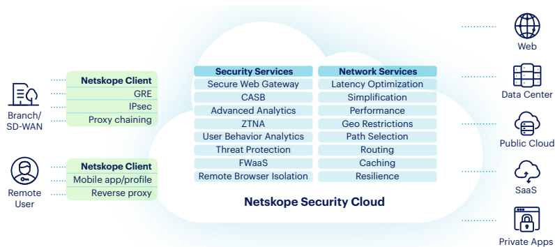
Figure 1: In addition to support for legacy proxies, firewalls, SD-WAN devices, and clientless options, Netskope Client simplifies steering traffic to Netskope NewEdge.
