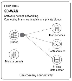
**FIGURE 1-2:** In the one-to-many world, the branch offices route traffic not just to the centralized data center using MPLS, but also to multiple clouds using MPLS and low-cost internet leveraging SD-WAN.
