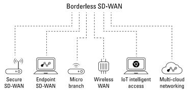
**FIGURE 2-1:** Borderless SD-WAN supports software on laptops, cellular gateways, and micro to large branch or data center appliances, and acts as a virtual gateway for multi-cloud networking.
