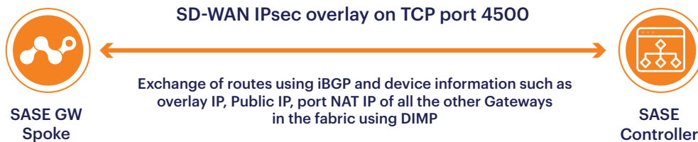
Figure 3: Routes and Device Information Exchange with Controller
